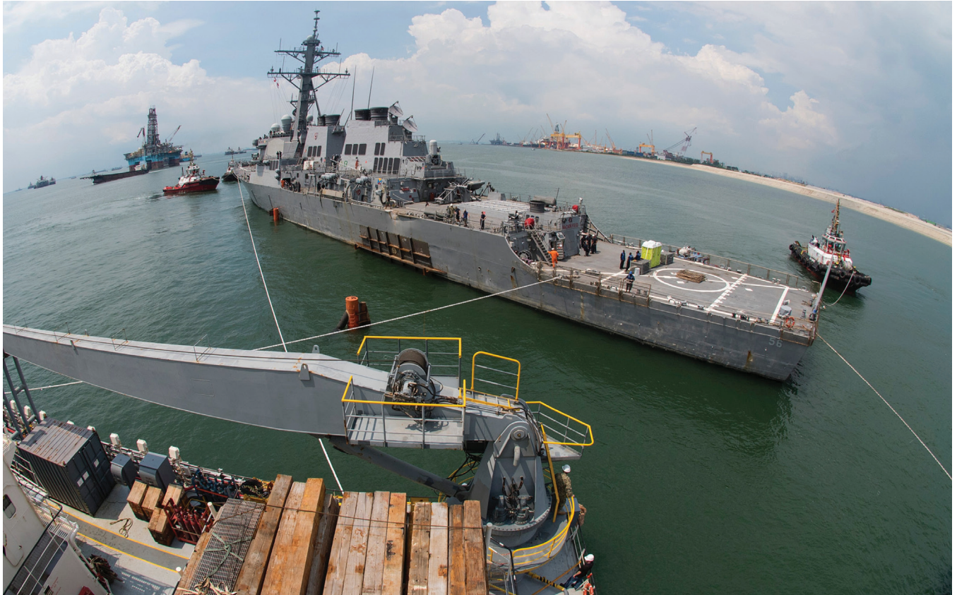
THE USS JOHN MCCAIN, DAMAGED in a collision with a merchant vessel in the Singapore Straits, is loaded onto a transport ship that will take the destroyer to Japan for repairs.
